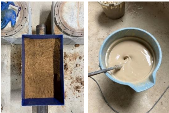
a) Testing sand b) Bentonite slurry
