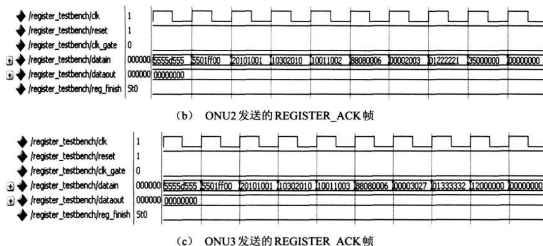
图7 ONU注册成功的确认结果图 Fig.7 Result confirming chart of successful ONU registration
