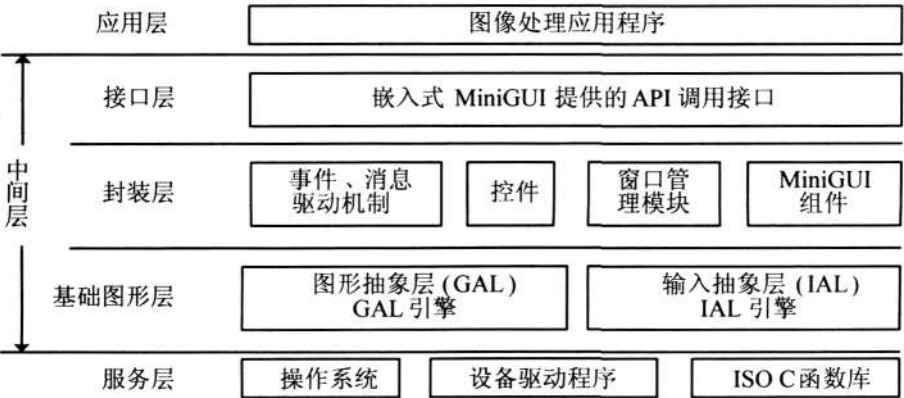
图3 嵌入式图像处理和GUI方案层次体系 Fig3. Embedded image processing and GUI program
