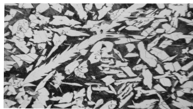
图9 边缘基体组织( \times 100 )4%硝酸酒精浸蚀 Fig.9 Matrix edge structure( \times 100 ), 4% nital etching
