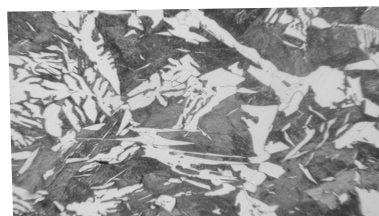
图8 中间基体组织( \times 100 )4%硝酸酒精浸蚀 Fig.8 Matrix middle structure( \times 100 ),4% nital etching
