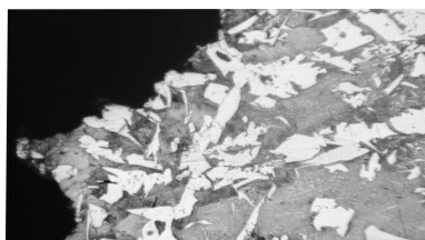
图7 断裂边缘组织( \times 100 )4%硝酸酒精浸蚀 Fig.7 Fracture edge structure( \times 100 ), 4% nital etching
