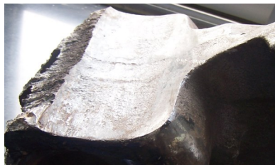
图1 发生断裂的钩舌 Fig.1 Coupler knuckle after fracture
