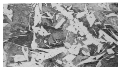
图10 中间背部基体组织( \times 100 )4%硝酸酒精浸蚀 Fig.10 Matrix middle-back structure( \times 100 ), 4% nital etching
