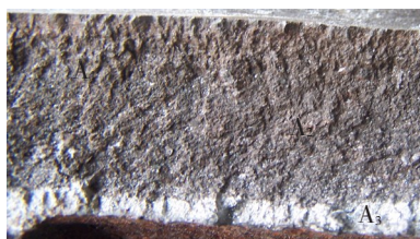
图3 钩舌A处的局部断口形貌 Fig.3 Local fracture surface of coupler knuckle A
