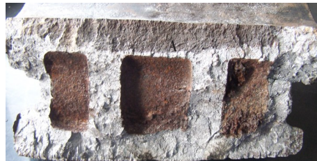
图2 钩舌的断口形貌 Fig.2 Fracture surface of the coupler knuckle
