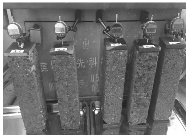
图 1 乳化沥青水泥稳定碎石干缩试验 Fig.1 Dry shrinkage test of emulsified asphalt cement stabilized macadam
