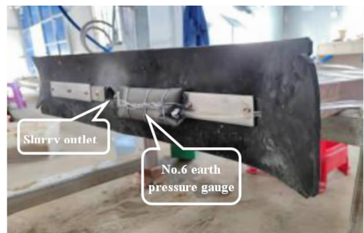
(b) Outlet pressure gauge position
