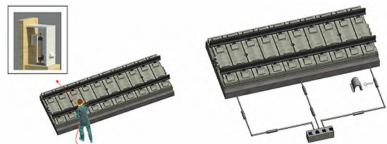
图6 安装流程模拟 Fig.6 Installation process simulation
