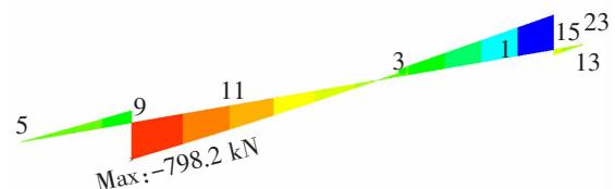
(b) Shear force  $F_z$  distribution diagram under combination condition 2
