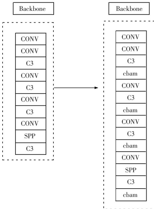
(a) CBAM-YOLOv5s-backbone algorithm
