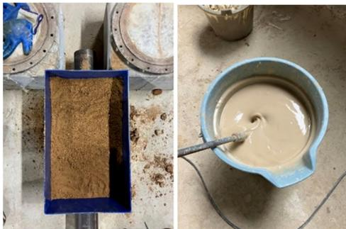
(a) Testing sand (b) Bentonite slurry
