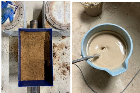
(a) Testing sand (b) Bentonite slurry
