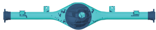
图1 桥壳网格质量检查结果 Fig. 1 Mesh quality inspection results of axle housing
