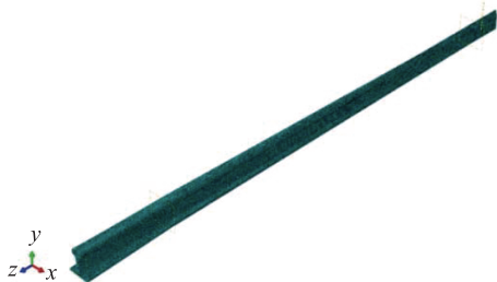
图1 道岔尖轨的三维有限元模型 Fig. 1 Three-dimensional finite element model of switch sharp rail
