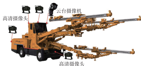
图7 三臂凿岩台车端主要硬件安装 Fig. 7 The main hardware installation on the three-arm rock drilling trolley
