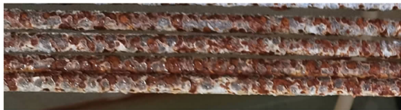
(c) Corrosion time 1 080 h
