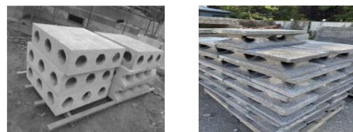
(a) Cross-shaped mould shell (b) Star mold shell
