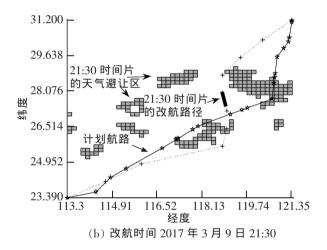
图 4 航迹随天气更新示意图 Fig.4 Tracks updated with different weather conditions over time
