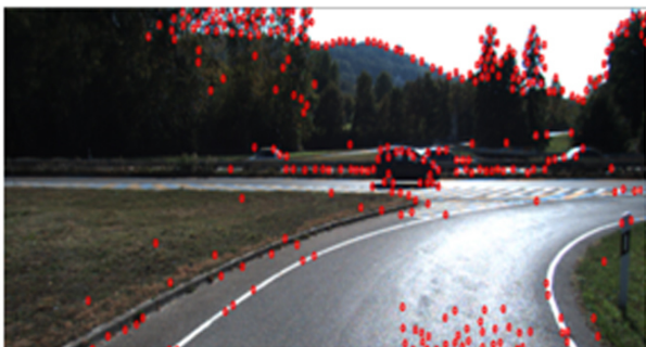
图 1 Shi-Tomasi 算法提取结果 Fig.1 Extraction result of Shi-Tomasi algorithm
