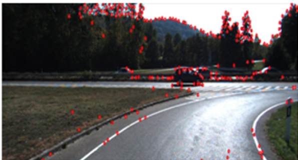
图 3 Harris 算法提取结果 Fig.3 Extraction results of Harris algorithm
