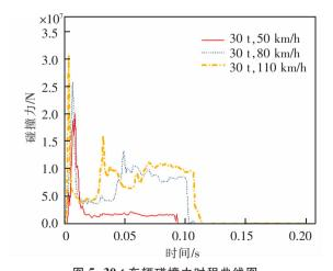
图 5 30 t 车辆碰撞力时程曲线图 Fig.5 Time history curve of 30 t vehicles of impacting force
