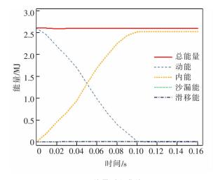
图 4 能量时程曲线 Fig.4 Time history curve of energy
