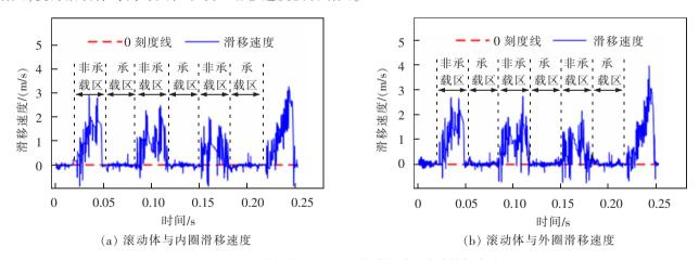
图 7 振幅为 5 000 N、振动频率为 100 Hz 轨道激励下滚动体与内外圈滑移速度 Fig.7 Sliding speed between rolling elements and raceways under orbital excitation with 5000 N amplitude and 100 Hz vibration frequency
