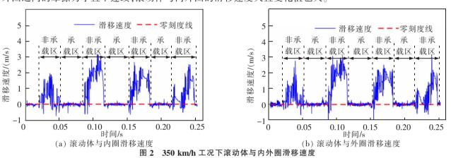
Fig.2 Sliding speed between rolling elements and raceways at 350 km/h
