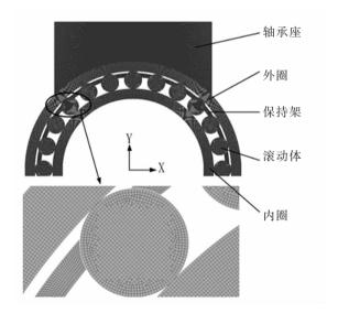
图 1 轴承及轴承座有限元模型 Fig.1 Finite element model of bearing and housing
