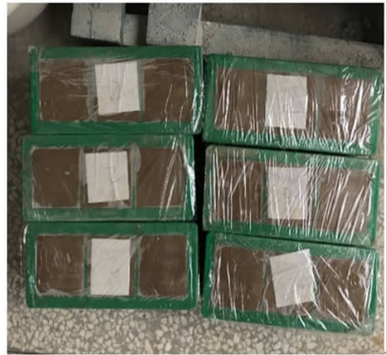
图 1 准备放入养护室的成型试件 Fig.1 Typical molded samples ready to be put into the curing room
