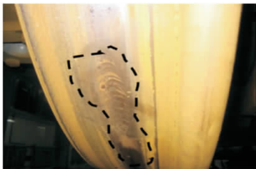
图1 车轮扁疤 Fig.1 Wheel flat
