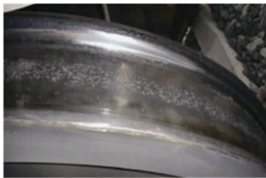
图2 车轮剥离 Fig.2 Wheel tread spalling
