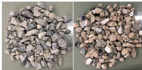
(a) Natural gravel (b) Ceramic coarse aggregate
