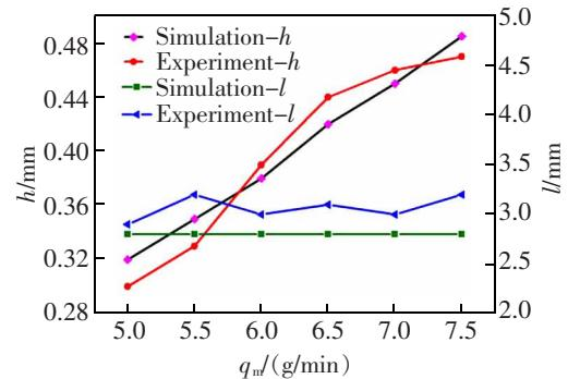
(a) Effect of the feeding rate on the size of the cladding layer
