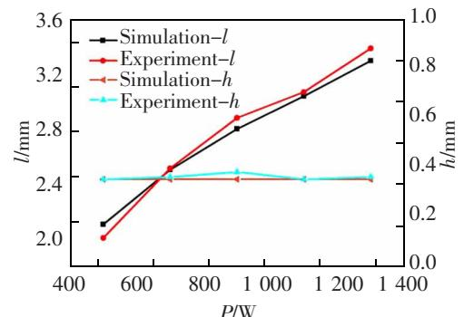
(b) Effect of laser power on the size of the cladding layer
