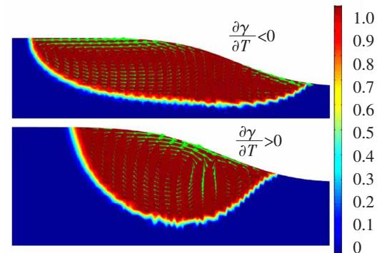
(b) Effect of surface tension coefficient on weld pool morphology
