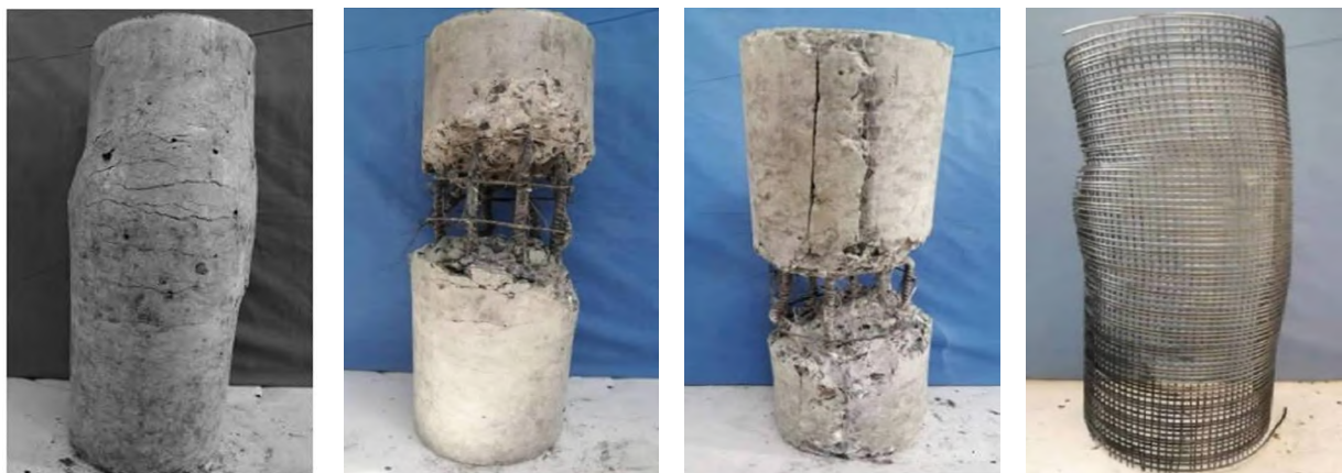
(a) Core concrete (b) Tension side reinforcement (c) Compression side reinforcement (d) Internal wire mesh
