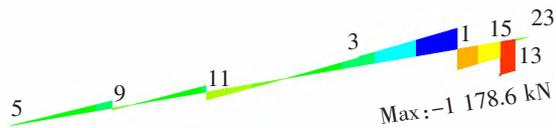
(b) Shear force  $F_z$  distribution diagram under combination condition 4
