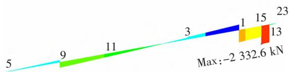
(b) Shear force  $F_z$  distribution diagram under combination condition 3
