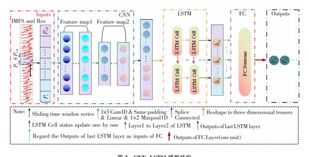
图 2 CNN-LSTM 模型结构 Fig.2 Structure of the CNN-LSTM model
