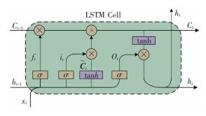
图 3 单个 LSTM 单元的内部结构 Fig.3 Internal structure of a single LSTM unit
